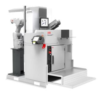
The FlexLoader<sup>™</sup> FP 300 is a standard equipment for automatic feeding of unsorted parts with a seeing robot. The equipment can separate and feed virtually all types of parts. Parts are poured out onto the FlexLoader<sup>™</sup> FP 300 buffer conveyor belt. Via different transport steps parts are separated onto the camera conveyor belt where a camera takes pictures.
